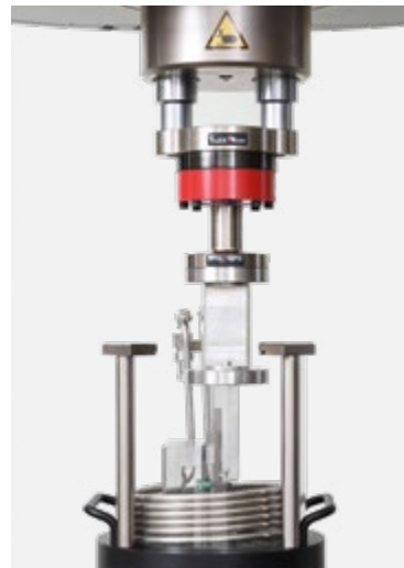
Test fixture for subassemblies to ASTM F1798 with temperature-controlled bath
