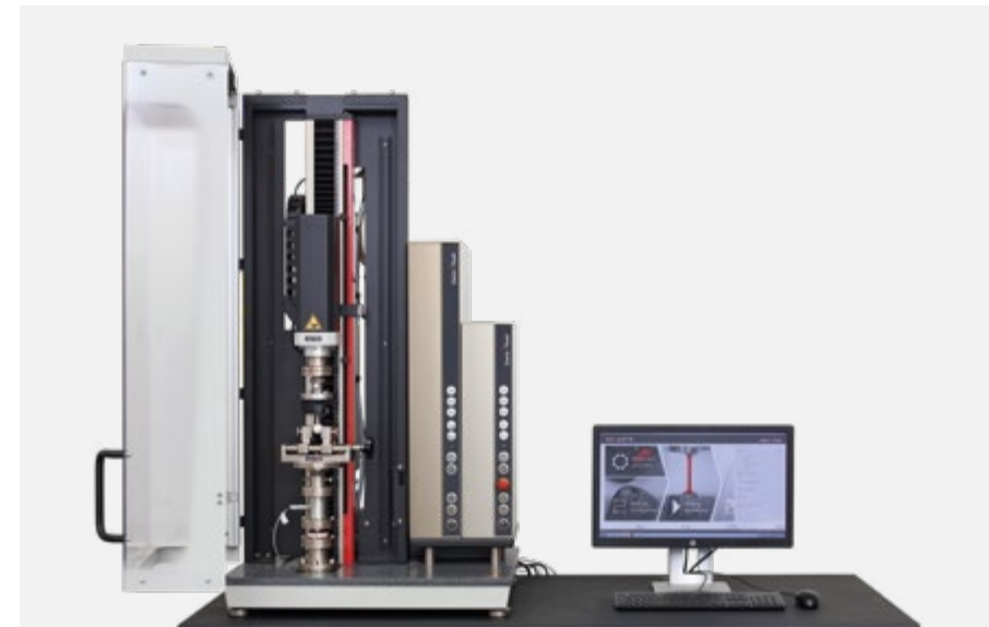
ZwickiLine Torsion testing machine for testing to ISO 7206-13
