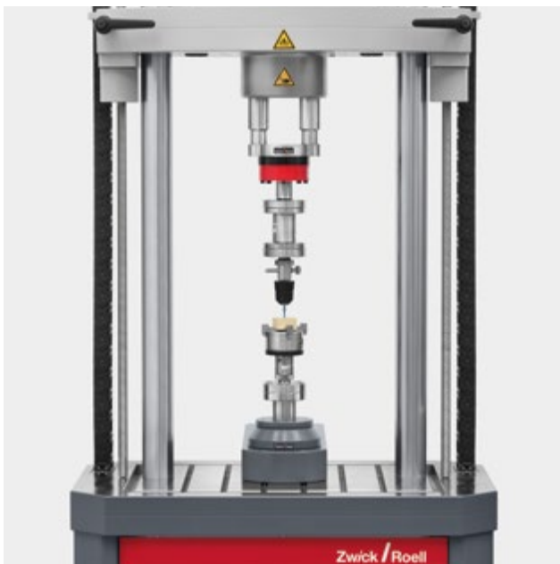
Testing of bone screws to ASTM F543 with an LTM electrodynamic testing machine
