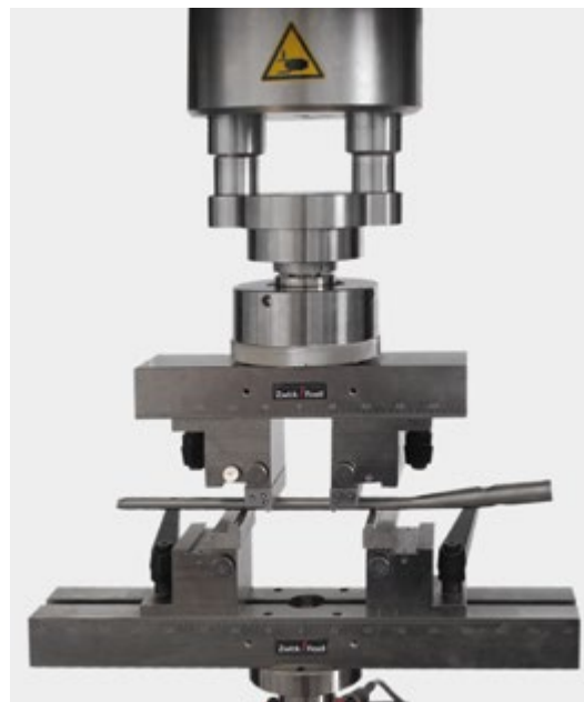
4-point flexure test kit for testing of bone pins to ASTM F1264
