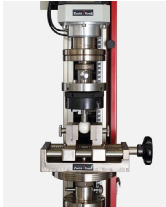
Test fixture for testing femoral heads to ISO 7206-13
