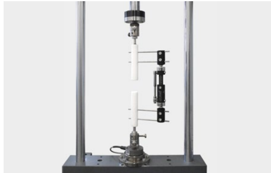
Test fixture for testing external fixation devices to ASTM F1541
