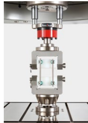
Test fixture for spinal implant constructs to ASTM F1717 and ASTM F2706
