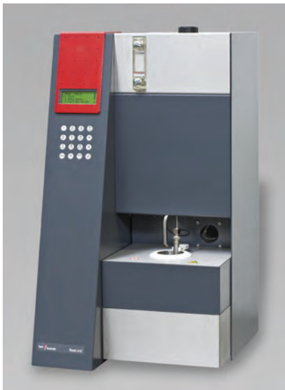
Fig. 1: ToniLIME instrument for determining free lime content
