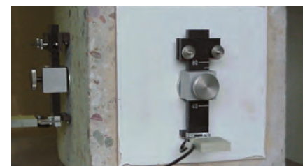
Fig. 3: Deformation transducer for the PCI test
