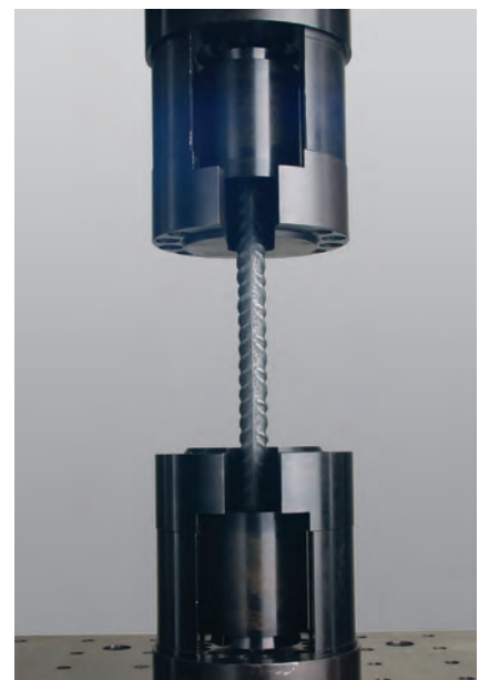
Fig. 4: Specimen grips and specimen embedding for ribbed rebar
