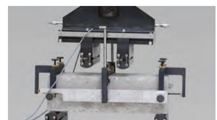
Fig. 4: Deformation transducer for measuring deflection
