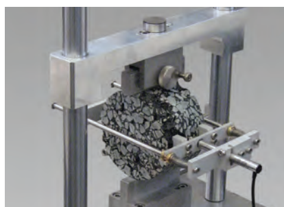
Fig. 2: Test device for uniaxial cyclic compression test
